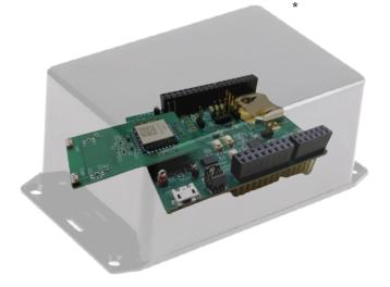
Flexible platform to develop customized UWB systems featuring **NXP's UWB chipset Trimension™ SR150**.
