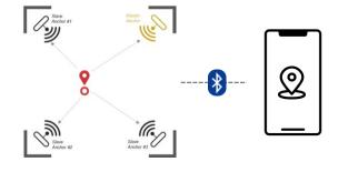
The **MK UWB RTLS Demo** showcases how UWB technology can be used to implement an uplink TDoA-based RTLS solution:
