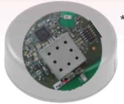
Autonomous, battery-powered UWB device that features **NXP's UWB chipset Trimention™ SR040** and a BLE-enabled microcontroller, enabling all kinds of tracking and localization use cases, including UWB RTLS tracking using TDoA multilateration.
