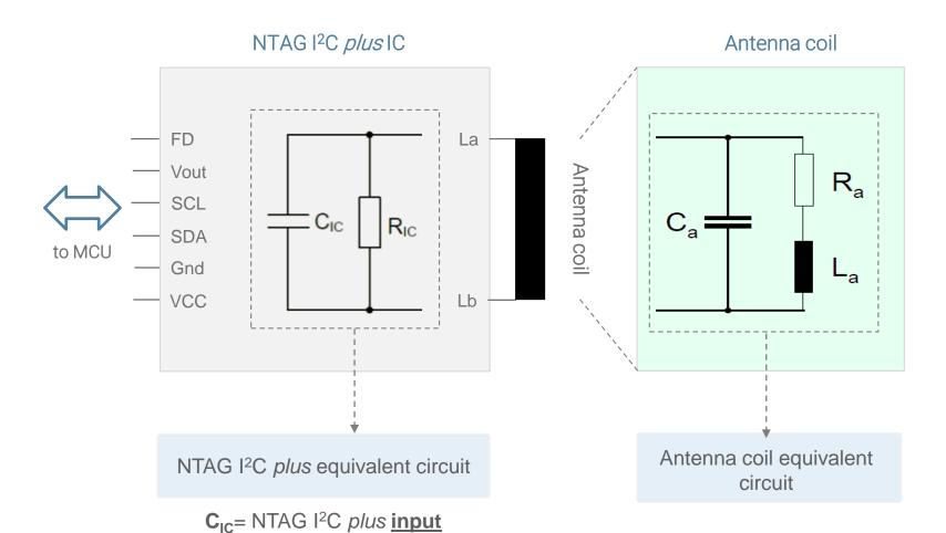
Each antenna is a resonant circuit with a specific input impedance.
