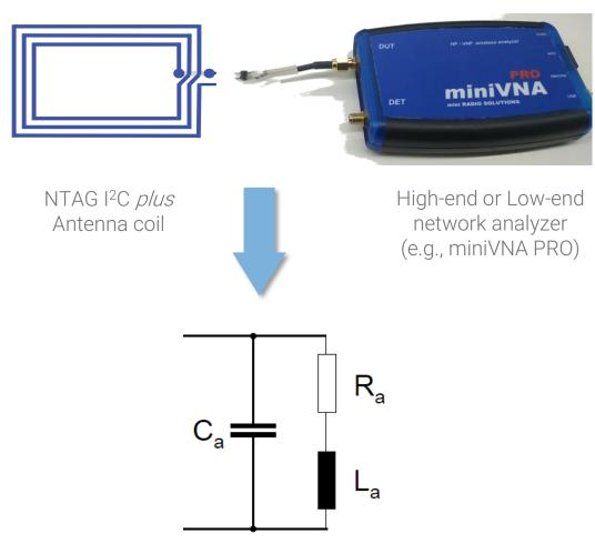
Fig. Antenna series equivalent circuit  $(C_a, L_a, R_a)$
