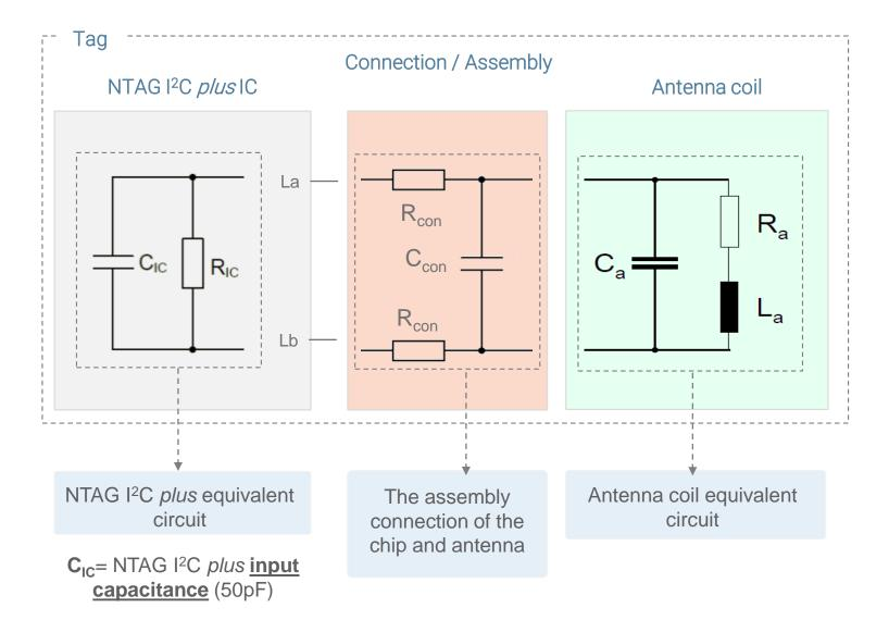
The resonance frequency of the tag can be calculated with:
