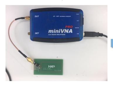
Fig 1. 54x27mm PCB antenna + NTAG I<sup>2</sup>C *plus* connected to miniVNA PRO
