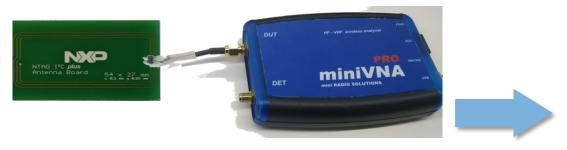
Fig 1. miniVNA PRO network analyzer connected to the 54x27mm PCB antenna connectors
