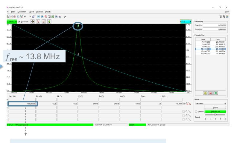
Good enough! If required, we can fine tune the capacitance until we reach the desired  $f_{res}$
