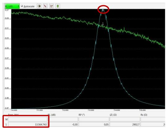
Fig. Example of a tag adjusted to  $f_{res} = 13.564 \text{ MHz}$
