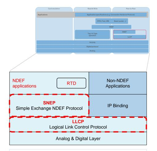
LLCP and SNEP enable the exchange of NDEF messages between NFC devices using P2P mode
