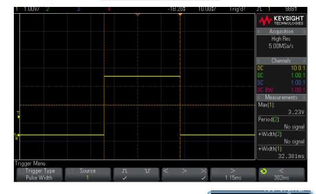
Measured time for a EMVCo loopback transaction takes **32ms**
