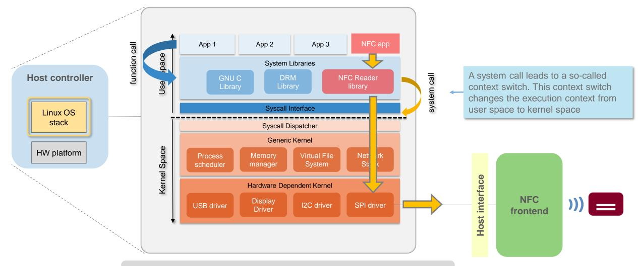
The NFC application needs to switch from User Space to Kernel Space for every SPI interface access
