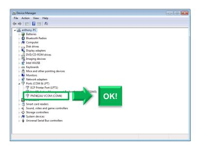
• If VCOM driver is not automatically installed, manually install it running with administrator rights <code>install\_vcom.bat</code>
