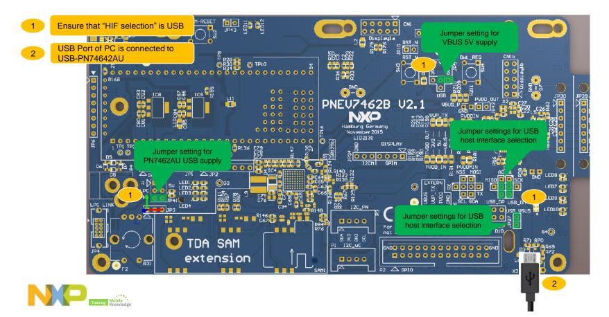
Step 3: Flash NFC Cockpit FW - Mounting USB as mass storage
