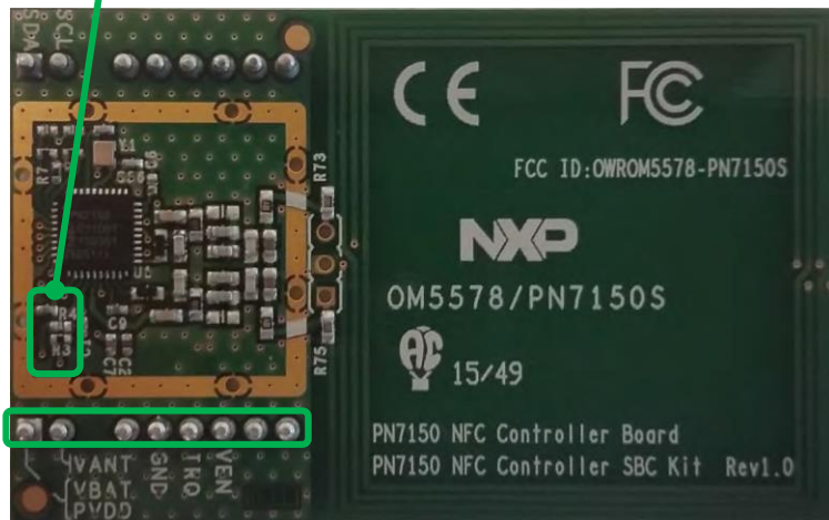
Fig. OM5578/PN7150S NFC controller board TVDD supply option
