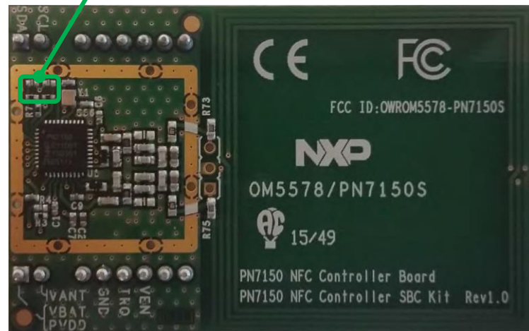
Fig. OM5578/PN7150S NFC controller board I2C address configuration
