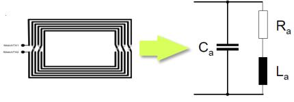
Fig. Antenna series equivalent circuit
